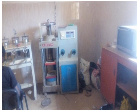
Plate 2: Flexural strength testing machine of 2000kN capacity
