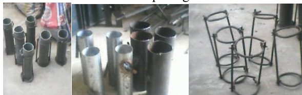
Plate 1: materials used for strengthening the openings
