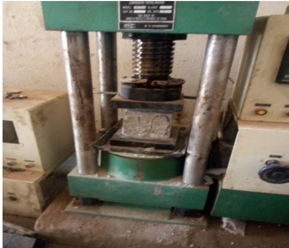
Figure 1: Specimen undergoing compressive strength test
