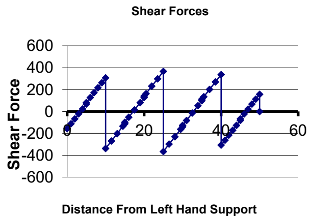
Figure 12: Shear Force (kN) Diagram for Exterior Main Girder
