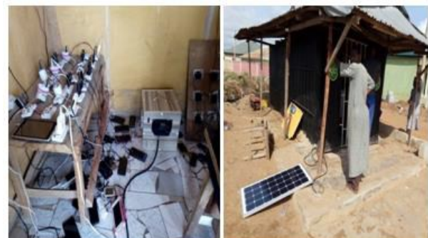
Figure 6: Deployment of NSEL solar mini generator at a mobile phone charging business center at Karshi, Nigeria (Mahmud, et al., 2020)
