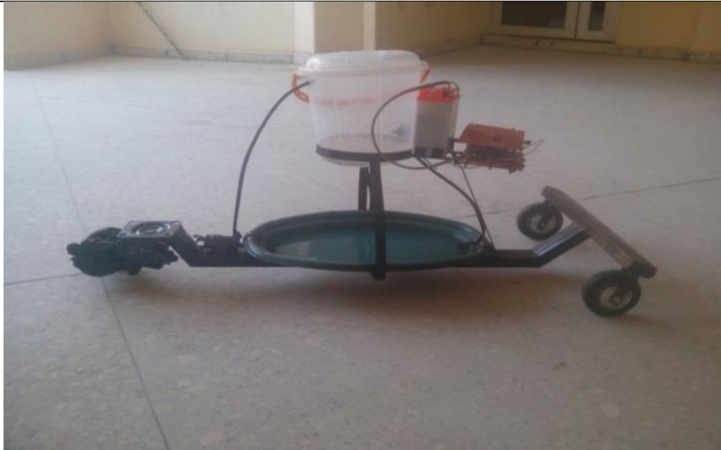
Figure 5: The final developed mobile intelligent liquid feed dispensing system
