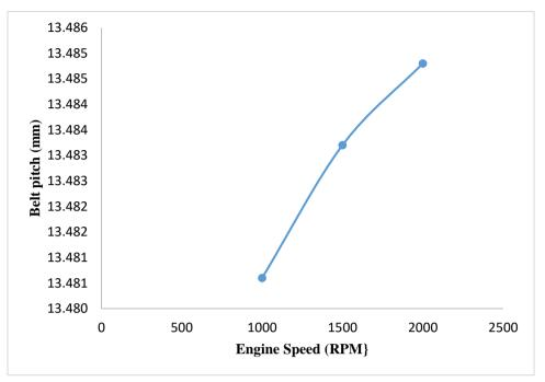
Figure 6: Effect of belt Pitch against Engine speed
