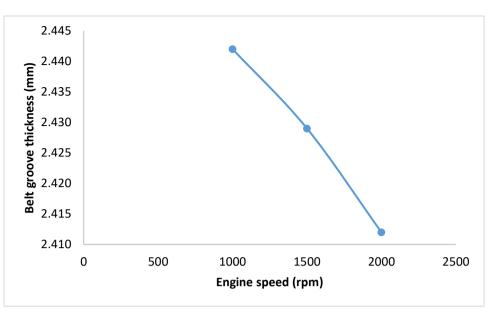
Figure 8: The effect of belt groove thickness against engine speed
