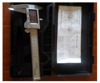
Figure 4: The Vanier Caliper
