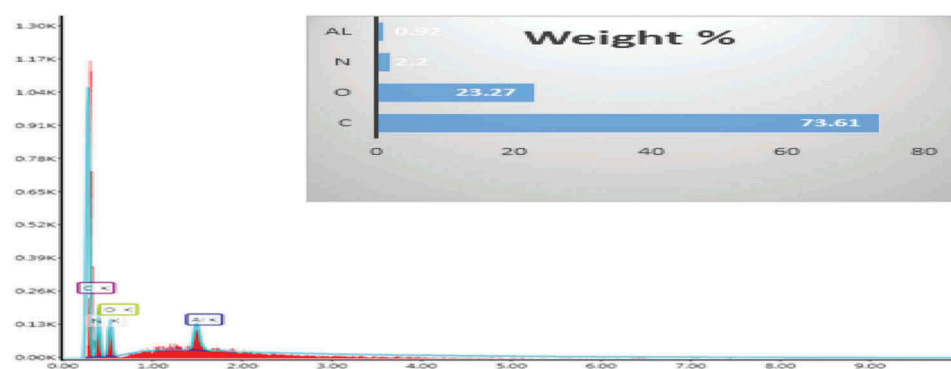
Figure 4. EDX spectra of CNS adsorbent (a) before adsorption and (b) after adsorption.
