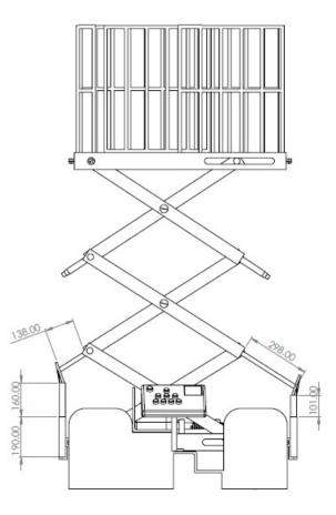
Figure 9: The full lift mode of the device on emergency support.
