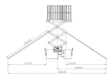
Figure 10: The full lift mode of the developed device with wind support arms deployed.
