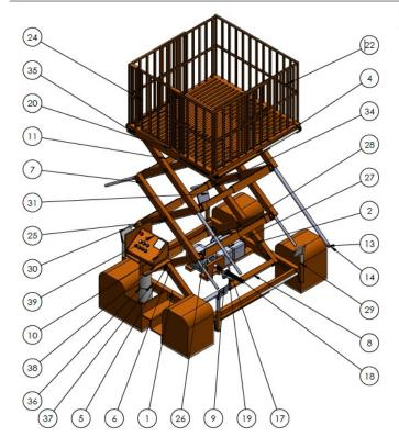
Figure 11: The part numbering of the designed scissor lifting model.
