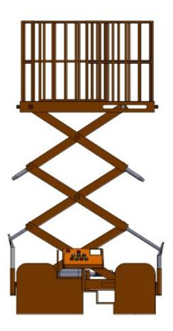
Figure 19: Side view of the designed improved intelligent mobile scissor lifting system.
