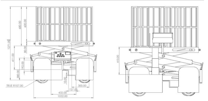
Figure 6: Front and side elevation of the improved intelligent mobile scissor lifting system on full collapse mode.
