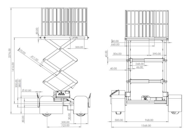
Figure 7: Front and side elevation of the improved intelligent mobile scissor lifting system on full lift mode. Table 2: The resistance-voltage relationship for distance determination.
