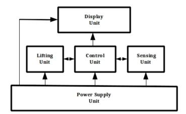
Figure 3: The block representation of the intelligent mobile scissor lifting model.
