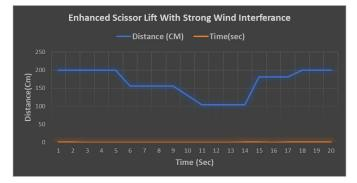
Figure 16: Results from the enhanced mobile scissor lifting system with strong wind effect.
