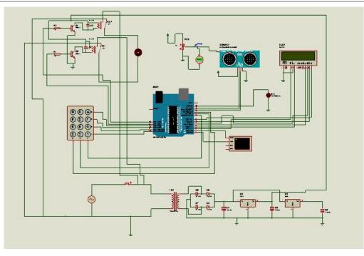
Figure 4: The electronic circuit for the intelligent mobile scissor lifting system .
