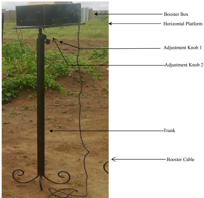
Plate III: A Booster Unit
