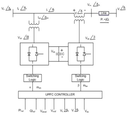
Figure 1. Block Diagram of a UPFC
