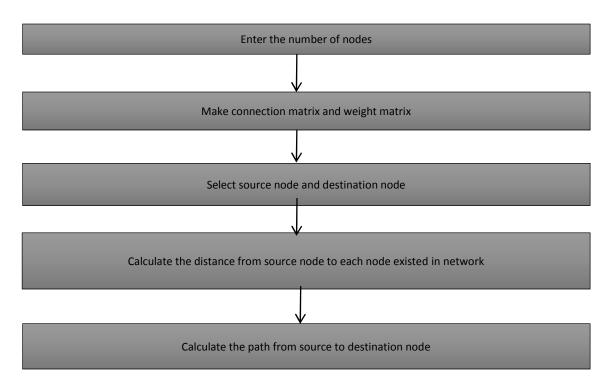
Figure 4 Dijkstra Flow Chart of Algorithm
