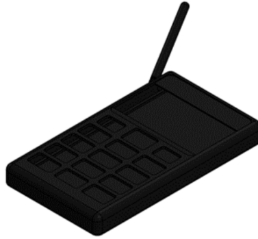
Figure 9: Assembled View of the Transceiver Package
