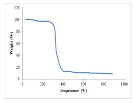
FIGURE 1: TGA THERMOGRAM OF RAW BAMBOO
