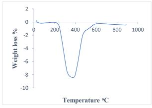
Figure 2: DTA properties of Lignite Coal
