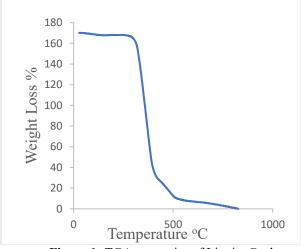
Figure 1: TGA properties of Lignite Coal
