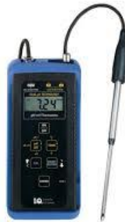
Figure 3-10 Photographic view of pH meter
