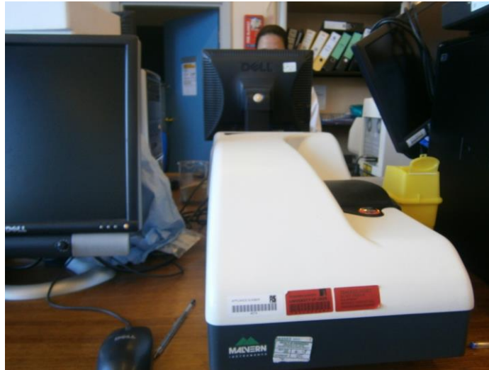
Figure 3-8 Photographic view of a Malvern 4800 zetasizer
