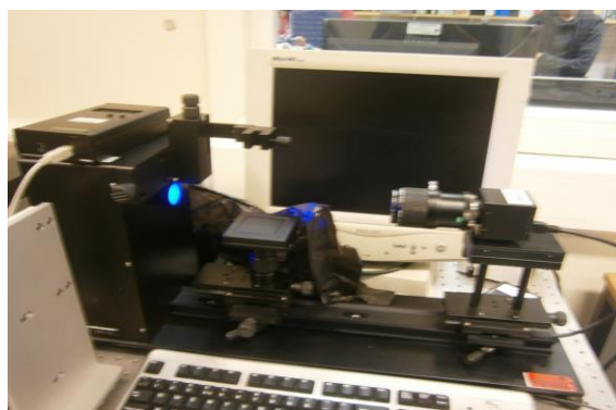
Figure 3-16 Photographic view of Attension Theta (Potential meter)
