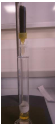
Figure 4-3 Laboratory clean-up experimental Set-up of oil contaminated soil using nano fluid
