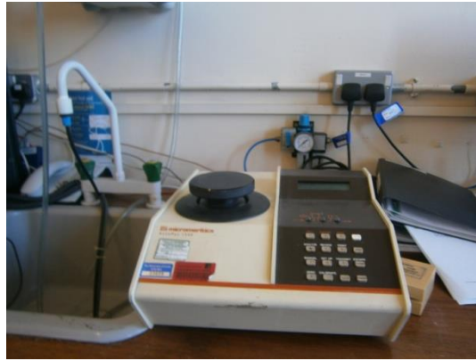
Figure 3-14 Photographic view of a Picnometer for measuring the density of mineral oil and nanofluids
