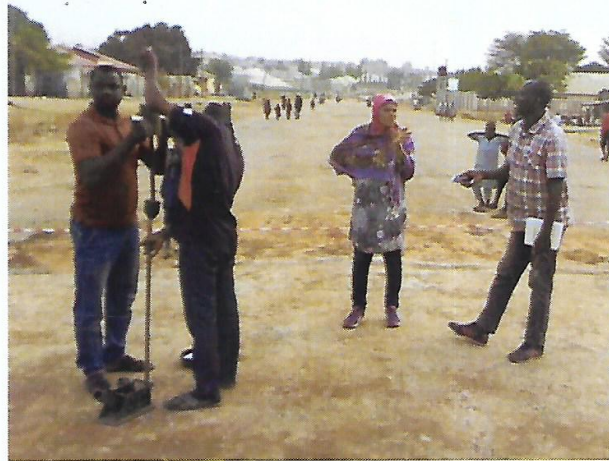
Figure 6: Dynamic cone penetration test to estimate CBR of the test sections
