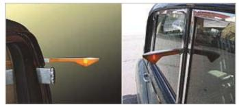
**Figure 1.** Trafficator in the "on" position **Source:** The free encyclopaedia
