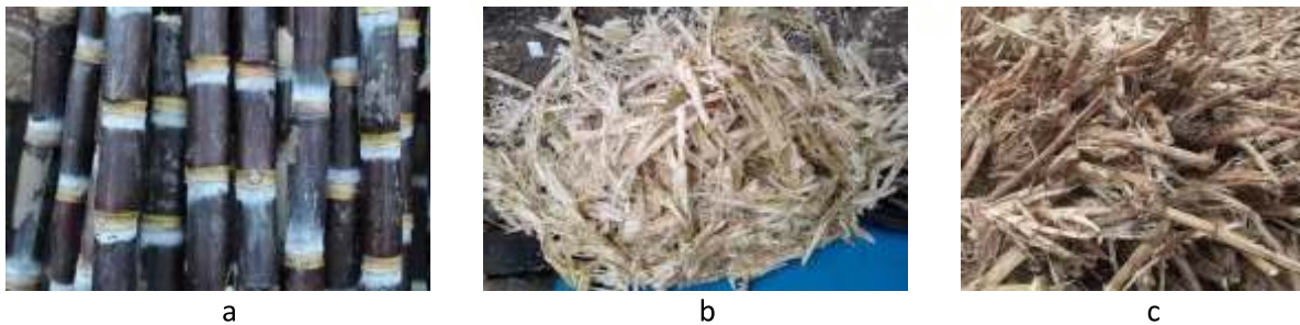
Figure 1: Sugarcane bagasse used: a) dark brown cover, b) inner whitish fibrous residue, c) combination of all parts of the sugarcane crop
