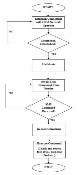
Figure 3: Flowchart of the GSM based remote monitoring and control system.
