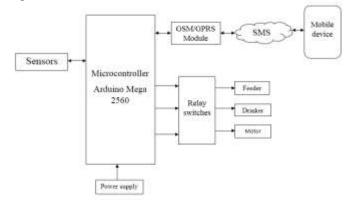
Figure 1: GSM based remote monitoring and control system
