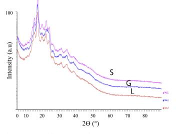
Fig. 1. X-ray powder diffraction patterns of Lagos (L), Giwa (G) and Sule (S) starches.
