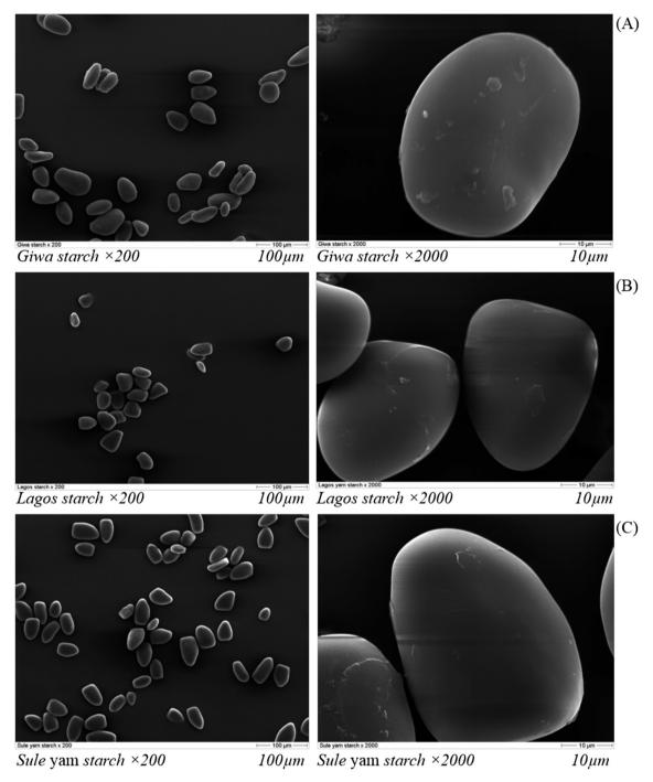
Fig. 2. Scanning electron microscope images (200x and 2,000x) of different cultivars of Dioscorea starches. (A) Giwa starch 200x, 100 µm and Giwa starch 2,000x, 10 µm; (B) Lagos starch 200x, 100 µm and Lagos starch 2000x, 10 µm; (C) Sule yam starch 200x, 100 µm and Sule yam starch 2000x, 10 µm.
