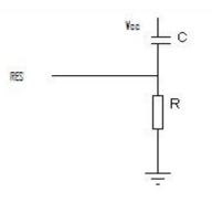
Figure 5.0: The Reset Circuit
