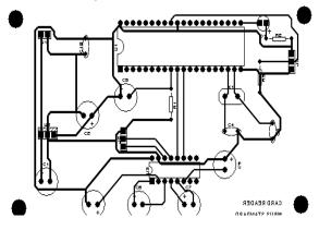
Figure 4.1 PCB Layout of the Card reader
