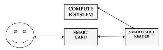
Figure 1.0: Block diagram of an Embedded Computer Based Lecture attendance system
