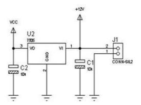
Figure 6.0: Three Terminal 7805 circuit for power protection
