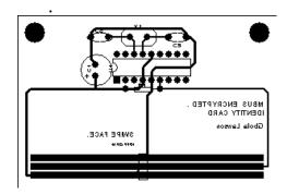
Figure 4.1 PCB Layout for card
