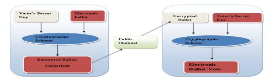
Figure 2: General Framework Cryptographic Model to Secure E-voting
