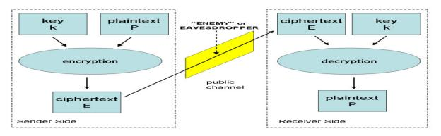
Fig 1: Symmetric-Key Cryptographic model (Source [14])
