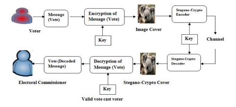
Figure 7: Stegano-Cryptographic Modeling Technique in Secure E-voting.
