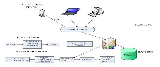
Figure 8: Architecture of the proposed model of Secured E-Voting System
