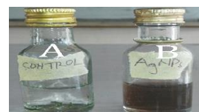
Figure 2: A, AgNO 3 as control; B, biosynthesized AgNPs after 30 minutes of bioreduction.
