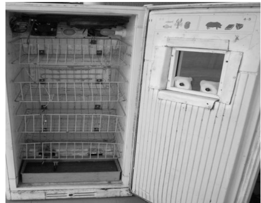
Figure 4 shows the embedded computer based incubator model
