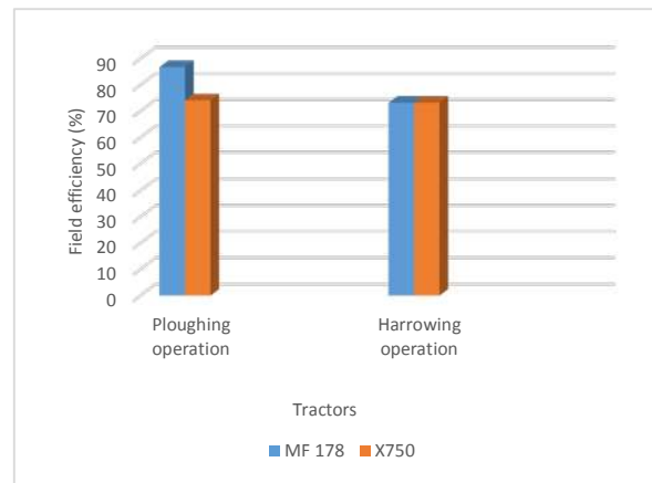
Fig. 9: Field efficiency of test tractors
