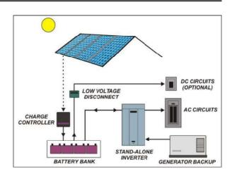
Figure 1: Off-grid PV System Schematic Source: Ammar & Noor (2018)
