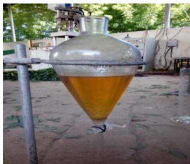
Figure 3: Separating process of essential oil and water
