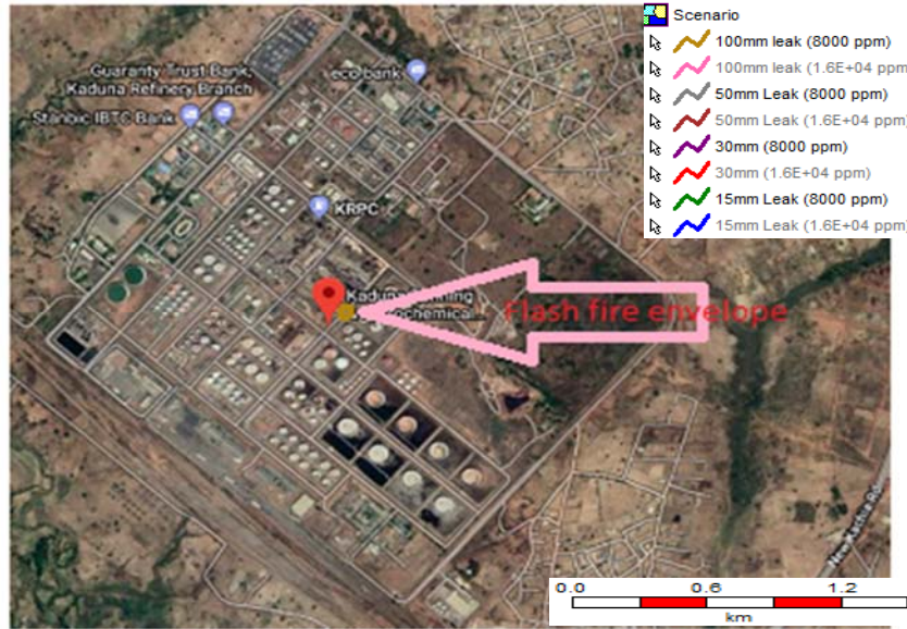
Plate I. 10H01 LPG Fuel Pipe Flash Fire Envelope
