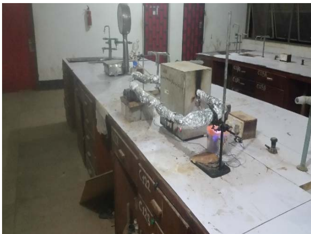
Plate I: Orthographic view of corrosion monitoring rig set-up.
