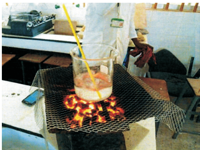
Fig. 6: Okaba coal combustion showing clean beaker with minimal smoke emission
