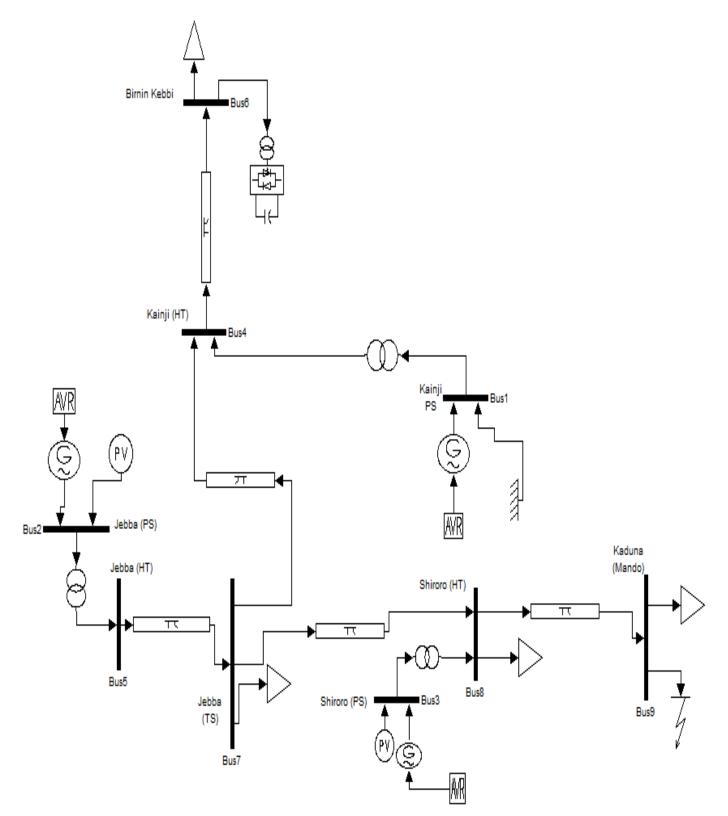
Figure 6. North-Central zone of the 330KV Nigeria grid system with STATCOM
