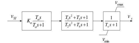
Figure 2. Power system stabilizer Type III
