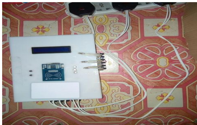
Plate I: Result showing connection to power supply
