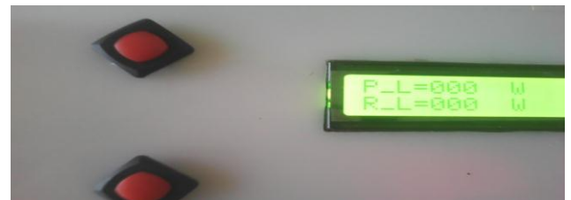
PLATE II: RESULT SHOWING THE CIRCUIT BREAKER READY TO BE PROGRAMMED TO DESIRED VALUES AND THE TWO BUTTONS USED TO PROGRAM IT.
