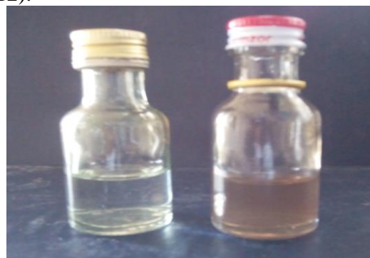
Fig. 2: Biosynthesized AgNPs (dark brown) using aqueous extract of wonderful kola after 15 min of reaction and the control AgNO 3 solution (colorless).
