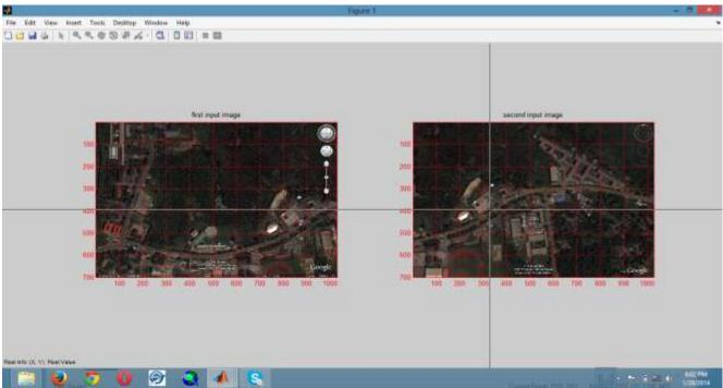
Figure 5.0a Showing the Process of Selecting Conjugate Points on both the Base (left) Moving and Moving Image
