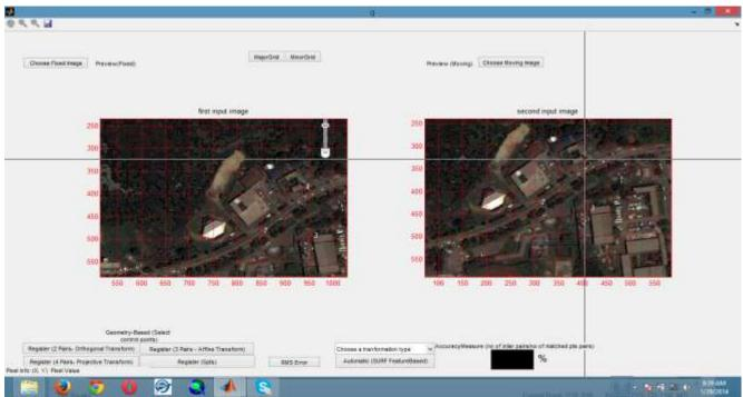
Figure 7.0a: Showing the Process of Selecting Conjugate Points on both the Base (left) Moving and Moving Image (Projective Transformation)
