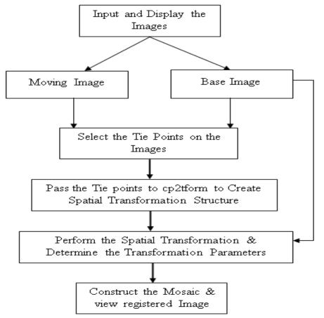
Figure 2.0: Flowchart showing the step by step procedure of carrying out a geometric (control point based) registration.
