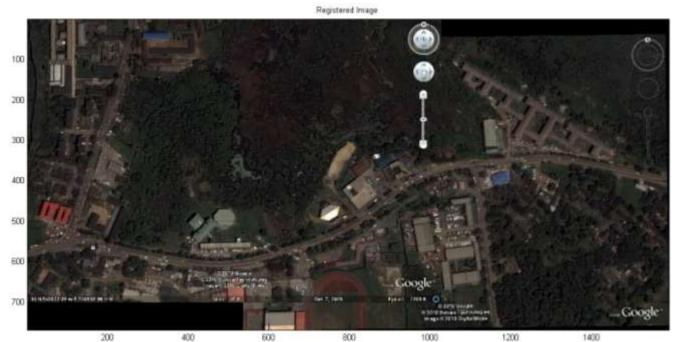
Figure 6.0b: Showing the Result obtained (registered image) using Affine transformation.
