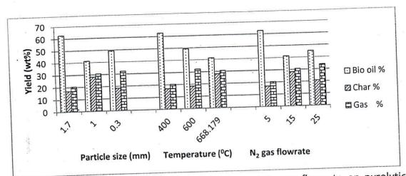
Chart 2: Effect of Particle size, Temperature and N2 gas flowrate on pyrolytic products Yield
