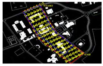
Figure 2: Mission's flight plan The image processing phase involves absolute orientation, relative orientation, and interior orientation. The procedure (Figure 3) involves camera calibration and alignment, point cloud and dense cloud generation, and DSM, DTM and DEM generation, and was performed using the Agisoft PhotoScan software which automatically generates large number of tie points based on Structure from Motion (SfM) algorithm.
