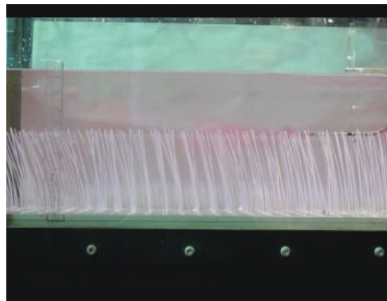
Figure 10. Physical modeling of flow over blade type vegetation.
