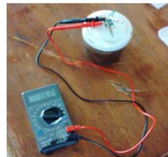
Plate 1 Voltage measurement from the MFC
