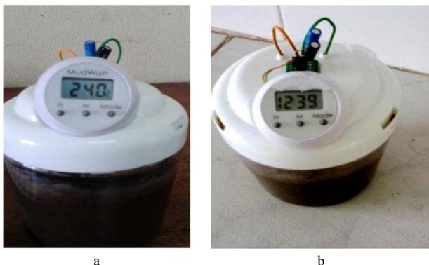
Plate 3 MFC<sub>urine</sub> powering (a) electronic clock (b) digital thermometer
