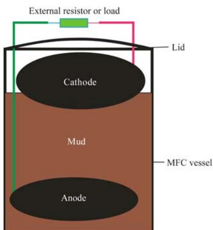
Figure 1 Schematic diagram of the MFC set-up
