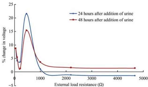
Figure 8 Percentage change in voltage across the external loads 24 hours and 48hours after urine addition to the MSCMFC
