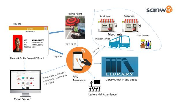
Figure 1: Flow process of the Sanwo's campus and city wide offline RFID based application
