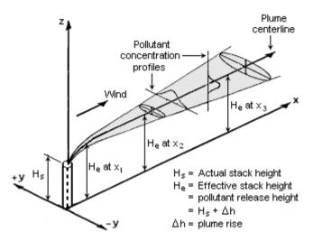
Figure 1: Visualisation of a bouyant Gaussian air dispersion plume in the atmosphere from a point emission source.
