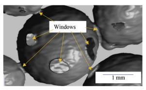
Fig. 1. Optical micrographs, left for a porous sample made by vacuum casting using near-spherical NaCl beads [10] and right, an X-ray CT image showing the typical pore connectivity [11].
