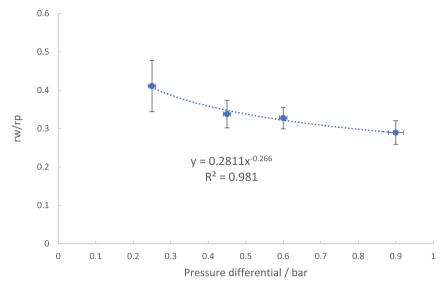
Fig. 7. Relationship between pressure differential and ratio of window to pore size for the cast samples.
