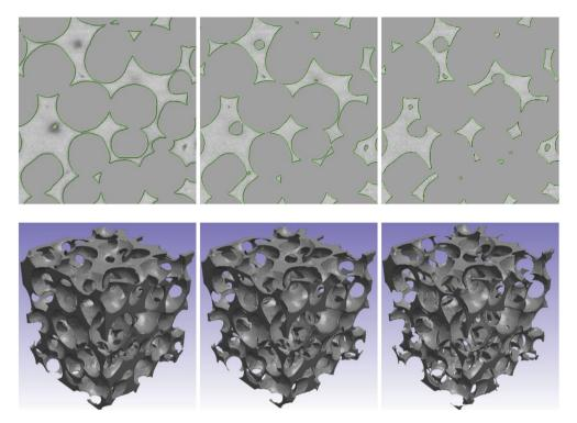
Fig. 11. 2D CT images (top) and 3D volumes (bottom) for sample P3 (left) and after erosion of 1 (centre, P31) and 2 (right, P32) pixels from the solid field (3D constructions are 8 × 8 × 8 mm).
