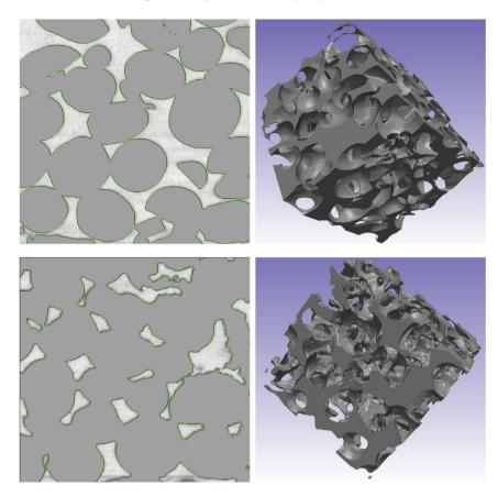
$\textbf{Fig. 6.} \ \ \text{Left, 2D model contours and right, metal domains for porous Al made at the highest (top) and lowest (bottom) pressure differentials (3D constructions are <math>8\times8\times8$  mm).}
