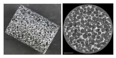
Fig. 5. 3D optical and corresponding 2D X-ray CT images of a porous Al structure (samples are 25 mm in diameter).
