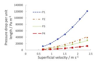
**Fig. 10.** Graph of measured (symbols) and modelled (dashed lines) pressure drops per unit length against superficial velocity.
