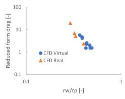
Fig. 12. Plots of the reduced permeability and form drag against the ratio of window to pore diameter for real and semi-virtual structures.
