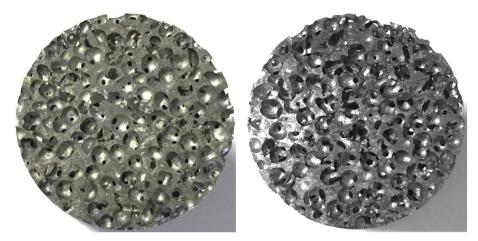
Fig. 4. Optical microscope images of porous Al foam structures made at (left) the highest and (right) the lowest pressure differential (samples are 25 mm in diameter).
