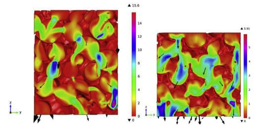
**Fig. 9.** 2D sections of the velocity distribution for flow through porous samples P1 (left) and P4 (right) for a superficial velocity of 1m s<sup>-1</sup> (RVE for P1 is  $8 \times 8 \times 10$  mm, for P4 it is  $8 \times 8 \times 8$  mm).
