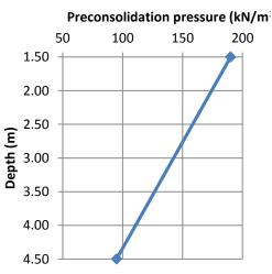
FIGURE 5: VARIATION OF PRECONSOLIDATION PRESSURE WITH DEPTH AT BH 4
