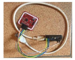
Figure 9 (a) Arduino interfaced with EHR system application (b) System NFC tag interface for modification (see online version for colours)
