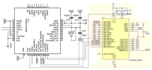
Figure 7 Circuit diagram of NFC based EHR authentication system (see online version for colours)
