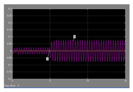
Figure 6. Results of angular vibrations of the sprung mass of the machine when moving on a sinusoidal surface (1-not shown, 2-passive springing, 3-active springing)
