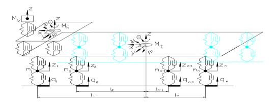
Figure 2-Spatial calculation scheme of transport vehicle vibrations
