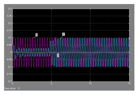
Figure 5. Results of movement of the machine's CM when moving on a sinusoidal surface (1perturbation, 2-passive springing, 3-active springing)
