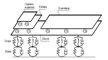
Figure 1-Generalized design scheme of a mobile object
