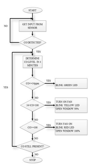
Fig. 7: Flow Diagram of the System
