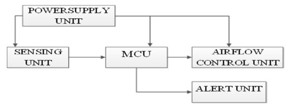
Fig. 1: Block Diagram of the CO Monitoring and Control System
