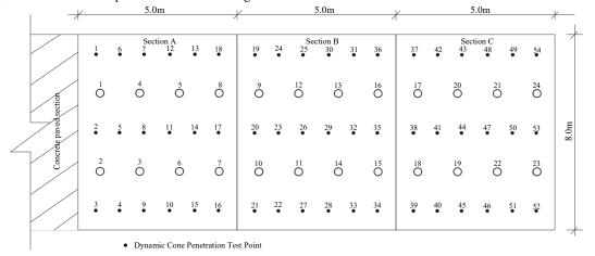
Fig. 5: Schematic diagram of the tested section of the road showing the tested points
