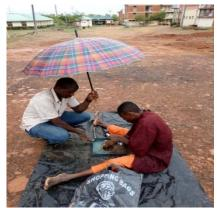
Fig. 10: In-situ density test on the road surface
