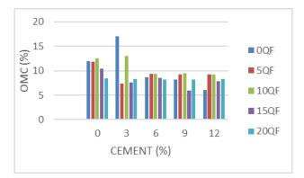
Fig. 4. Effect of Quarry Fines and Cement on Optimum Moisture Content
