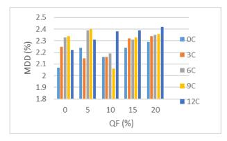
FIGURE 3: EFFECT OF QUARRY FINES AND CEMENT ON MAXIMUM DRY DENSITY
