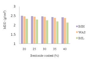
FIGURE 3: EFFECT OF BENTONITE CONTENT ON MDD OF MIXTURES.
