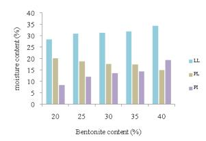
FIGURE 2: VARIATION OF CONSISTENCY LIMITS WITH BENTONITE CONTENT
