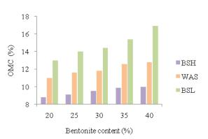
FIGURE 4: EFFECT OF BENTONITE CONTENT ON OMC OF MIXTURES
