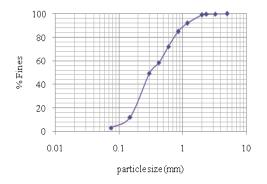
FIGURE 1: PARTICLE SIZE DISTRIBUTION CURVE (IOT)
