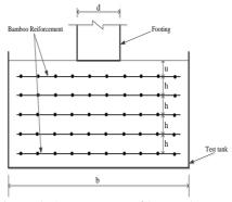
Figure 4: Arrangement of layers the bamboo reinforcement
