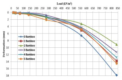
Figure 6: Load-settlement test result
