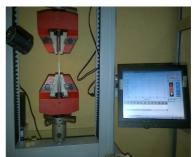
Figure 2: Bamboo splint in tension
