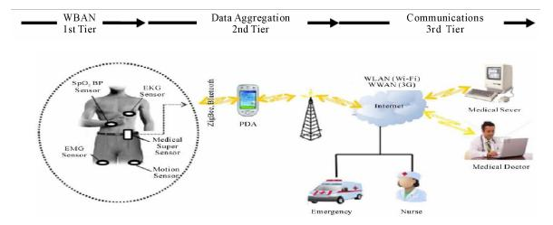
Figure 1: Generic Architecture of wireless sensor networks for remote healthcare monitoring system [13]
