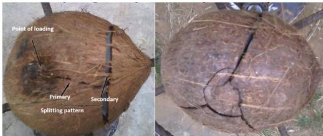
Figure 3: Punch-splitting by the machine
