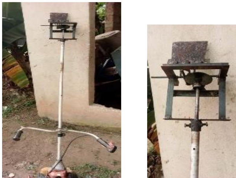
Plate 1: Motorized palm fruit harvester with a scotch yoke mechanism
