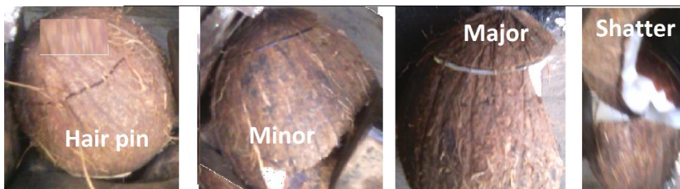
Figure 6: Pattern of cracks on coconut samples
