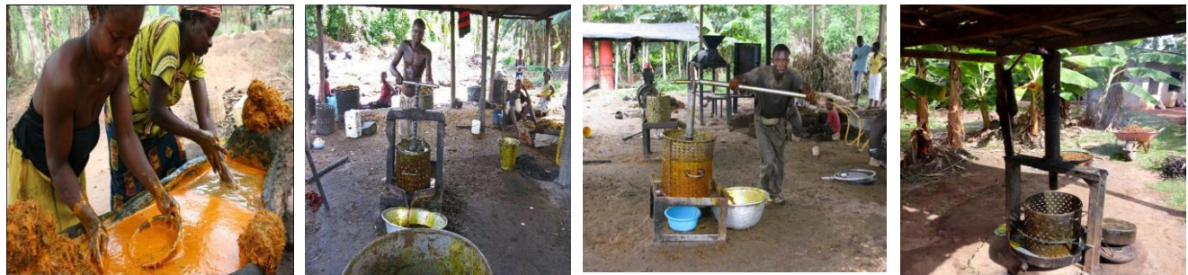
(a) Traditional method of extracting palm oil. (b) A manual screw press operator at work. (c) A long manual screw press operator at work. (d) A manual spindle press.
