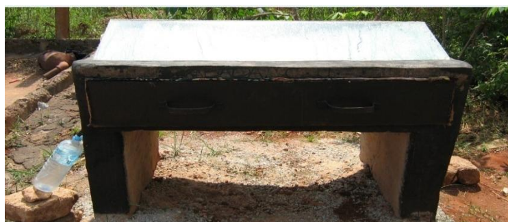
Fig. 3: The Newly Developed Solar Desalination System.
