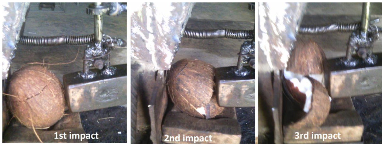
Figure 4: Impact-splitting action of the machine
