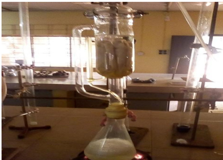
Fig.3: Experimental set up of the solvent extraction method of moringa seed Some portion containing the solvent then recycled back to the round bottom flask as it refluxed and the total process of reflux continues until all oil was extracted. This process was repeated for 5 more runs of the sample to expel all the oil. Proximate analysis was carried out according to the procedure of Association of Official Analytical Chemist (AOAC, 1990) to determine the moisture content, crude fiber, protein, crude fat, and carbohydrate components of the seed oil.
