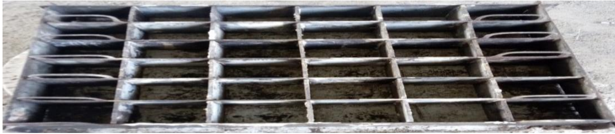
Figure 1. Moulds Specially Fabricated for Cube Production
