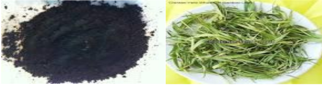
Fig.1 (a) BLA after incineration and sieving. (b) BLA in wet purchased condition .
