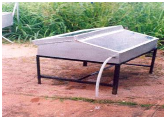
Fig 2: Picture of earlier designed solar still. Source: (Ogwo 2005)
