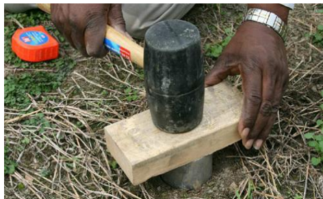
Plate 1: A three inch diameter ring is hammered into the soil to collect bulk density samples Source: (Arshad, 1996)
