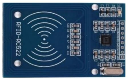
Figure 2: RFID Reader (Robomart, 2015)
