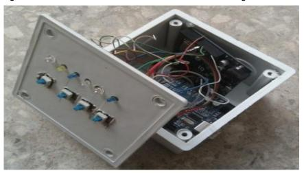
Figure 17: Developed Wireless RFID Reader
