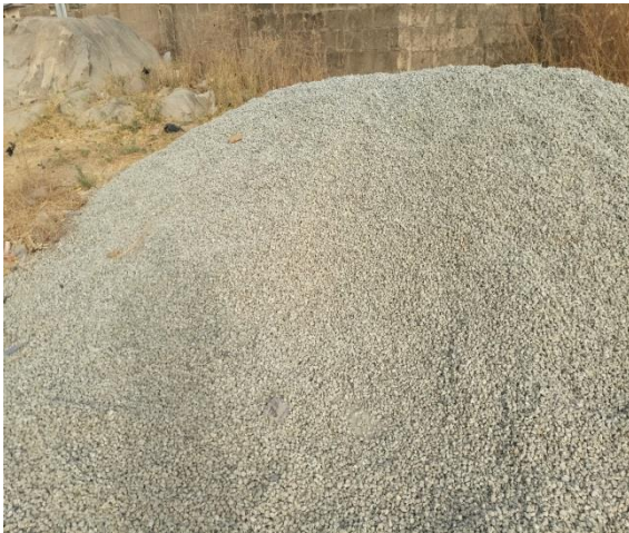
Plate IV. Granite Chippings for gravel packing. Plate V. Inappropriate Gravel packing of a borehole
