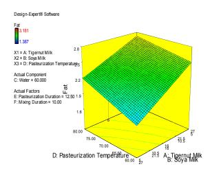
Fig. 8: 3 D Surface Mix-Process Plots Showing the Effect of Pasteurization Temperature on the Yield of Fat with Respect to the Milk Composition.
